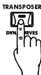
1. Press the **[TRANPOSE]** button and keep it pressed for at least two seconds. The LED will begin to flash.
