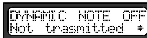
This function allows to send or not the MIDI code of the Note Off Velocity.
