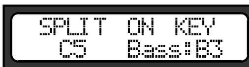
The cursor will move to parameter B4, which is the factory set (default) split point (this means that from C $\emptyset$  to B3 a bass voice can be played with, for example, a piano voice from C4 to G9).
