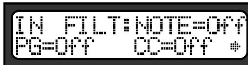
The **IN FILTER** function allows you to “filter” certain information entering the instrument. The NOTE, PROGRAM CHANGE (PG) and CONTROL CHANGE (CC) field in the **IN FILTER** function can be enabled or disabled.
