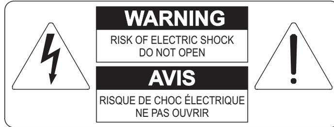
This symbol is intended to alert the user to the presence of uninsulated “dangerous voltage” within the product’s enclosure that may be of sufficient magnitude to constitute a risk of electric shock to persons.
